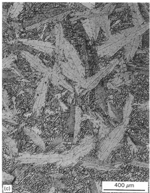
Figure 4 Optical micrographs of the etched surface of sintered SiC. Sintering temperature: (a) 2223 K, (b) 2273 K and (c) 2323 K.
